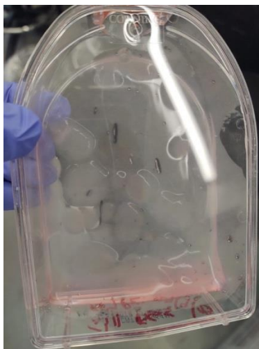
Figure 37 is a photograph showing an example T75 culture flask containing FBS-cultured ADSCs, which is contaminated with fungus.
