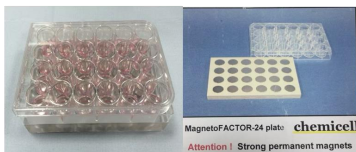
Figure 39 illustrates the experimental setup of SPION-labelling cells in a 24-well plate with a MagnetoFACTOR-24 device (Chemicell).
