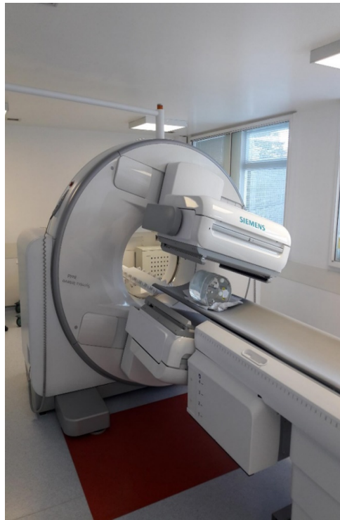
Figure 2.1: Example of a modern SPECT-CT gamma camera: a Siemens Intevo Bold (Siemens Healthineers, Erlangen Germany).
