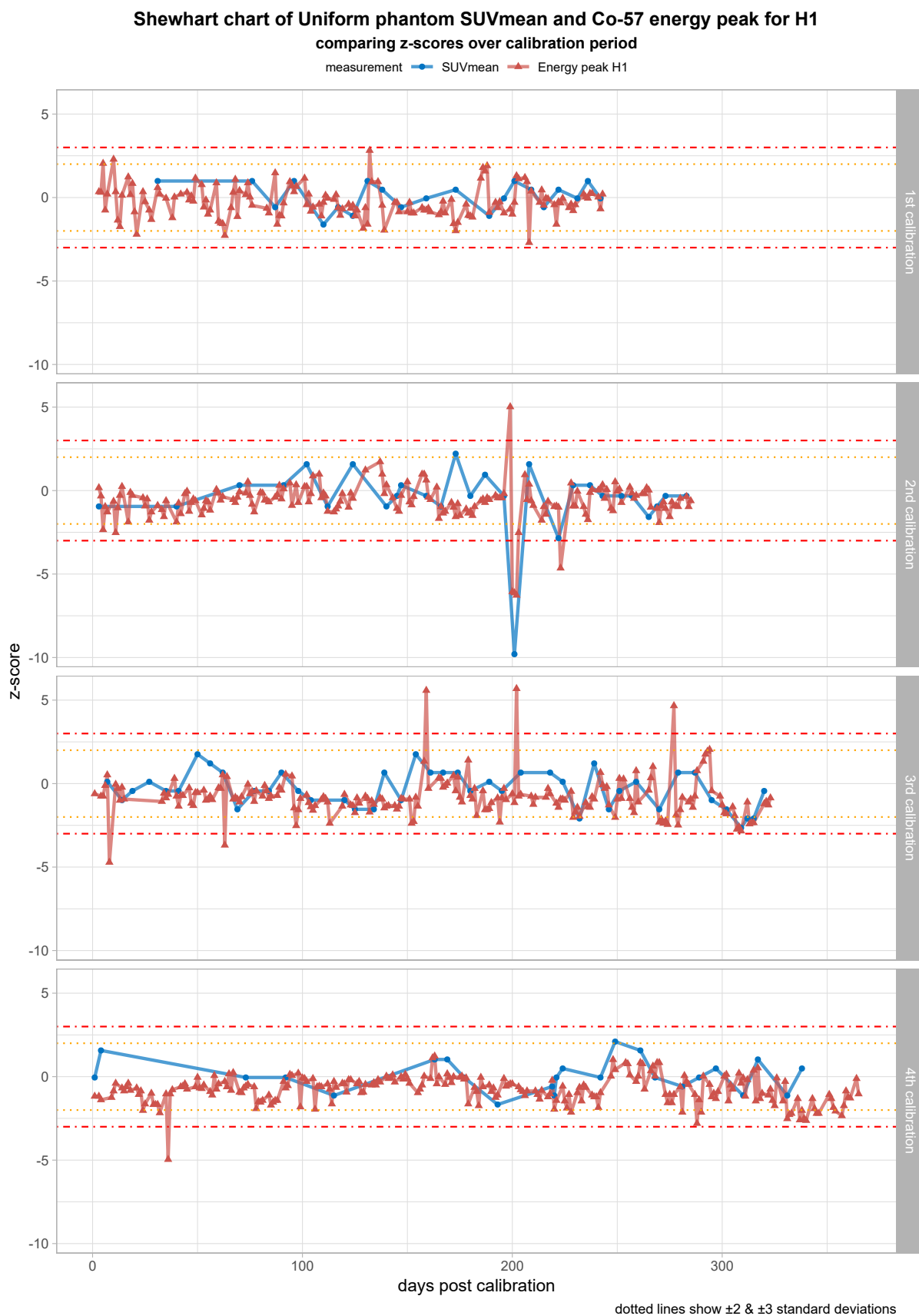
Figure 7.21: Comparison of longitudinal ^{99m}\text{Tc} SUV measurements with ^{57}\text{Co} energy peak deviation, for detector head 1
