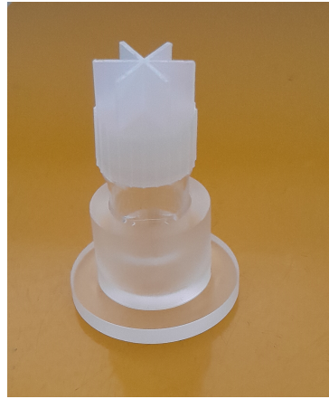
Figure 6.4: Positioning jig (designed and manufactured for this thesis) to allow reproducible positioning of point source within calibrator dipper.
