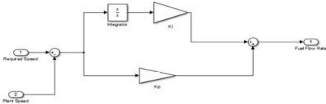
Figure 4.5: Model inside subsystem of Simulink model
