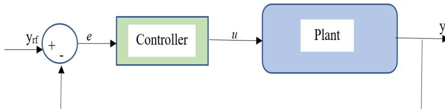
Figure 4.1: Block diagram of a process with a feedback controller
