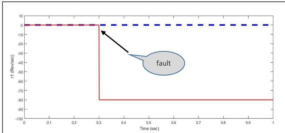
Figure 5.3: Residual plot of  $r1$ (spool speed) in case of  $f1$
