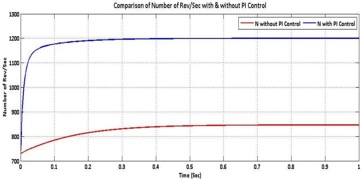
Figure 4.6: Plot showing RPM control by PI Controller
