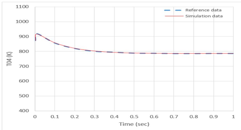
Figure 3.8 (b): Validation of model in case of turbine exit temperature
