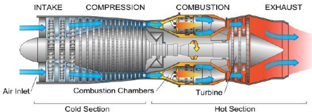
Figure 2.1: Single-shaft gas turbine engine (Asgari, 2014; 2016)
