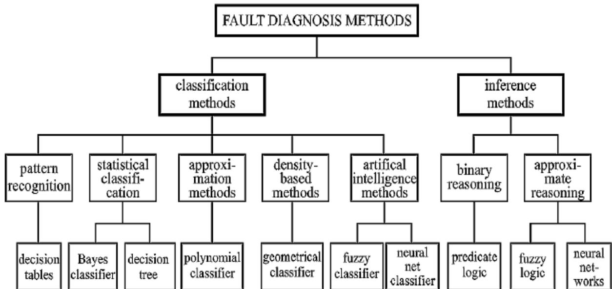
Figure 2.3: Survey on fault diagnosis methods (Isermann, 2006)
