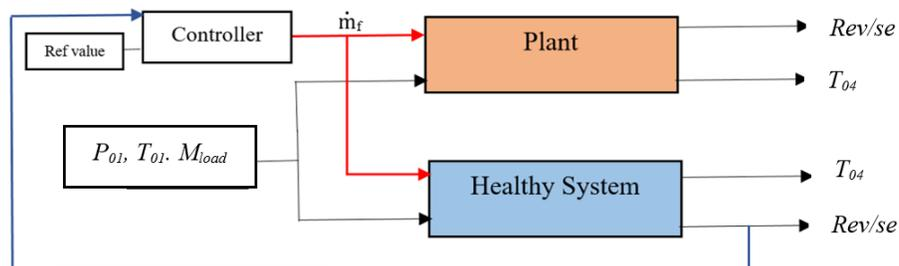
Figure 5.15: Model for recovery from RPM sensor fault in gas turbine
