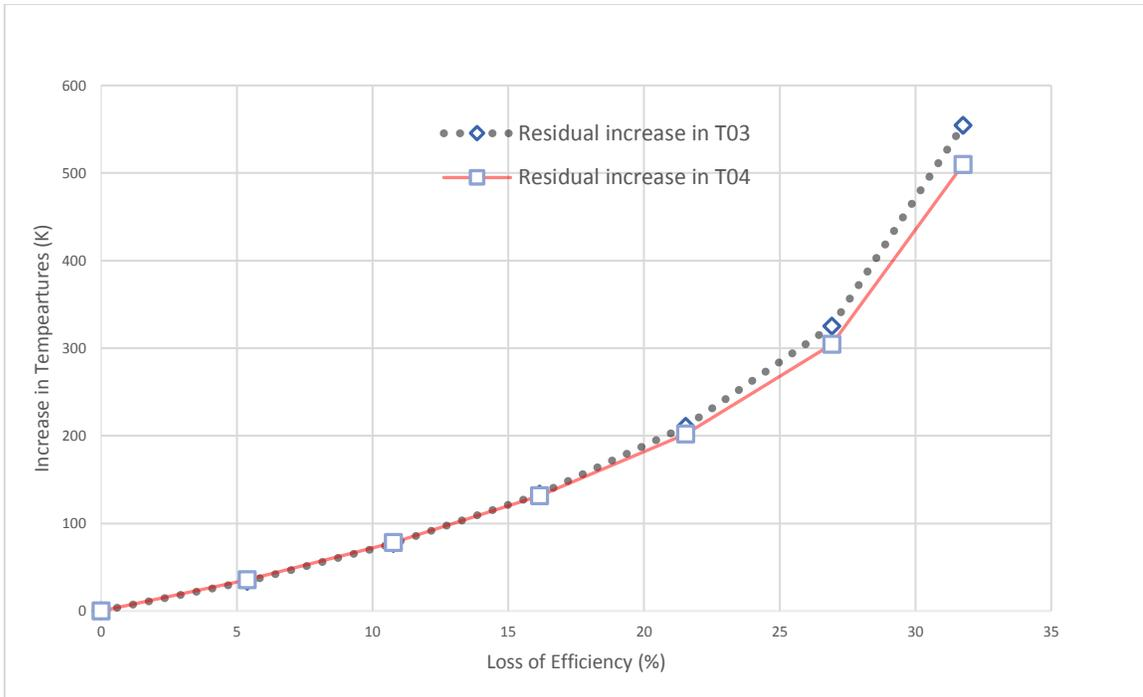
Figure 5.13: Increase in temperatures in case of FOD
