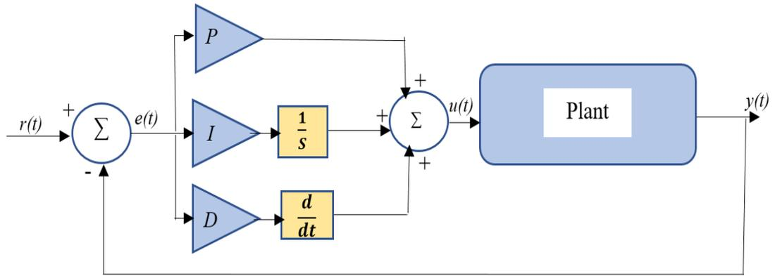
Figure 4.2: PID control structure
