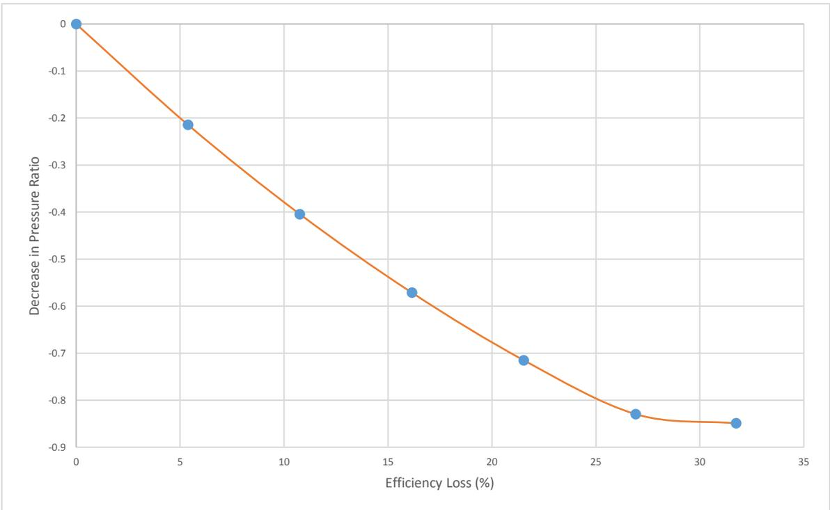
Figure 5.14: Decrease in compressor pressure ratio in case of efficiency loss
