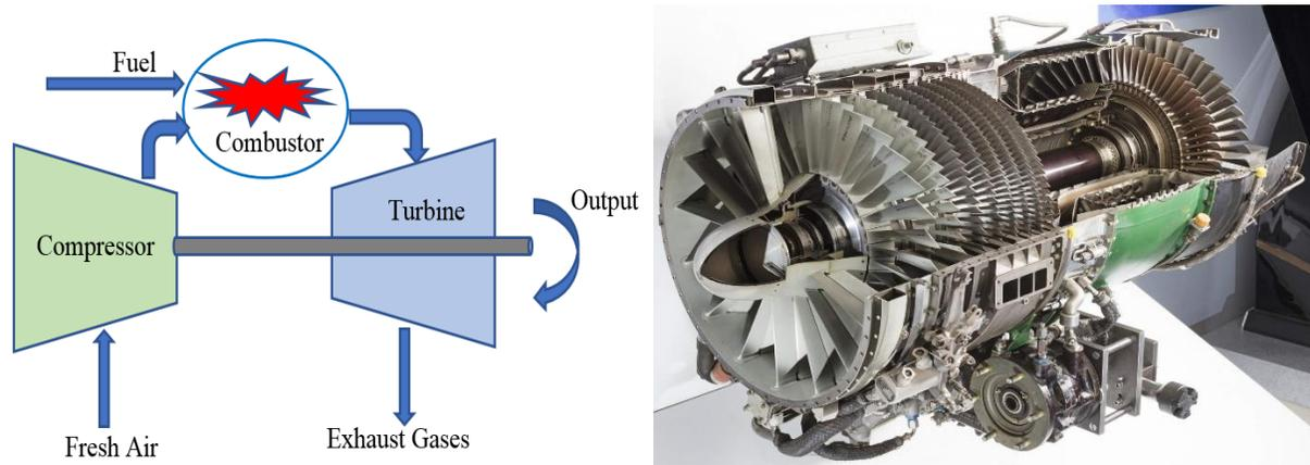
*Figure 1.1: Basic operation of the gas turbine engine*
