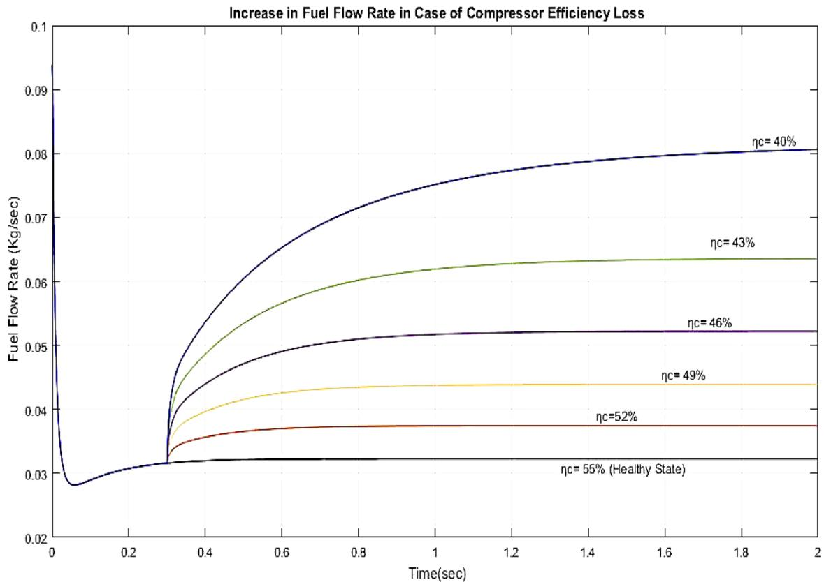
Figure 5.12: Rise in fuel flow rate in case of compressor efficiency loss
