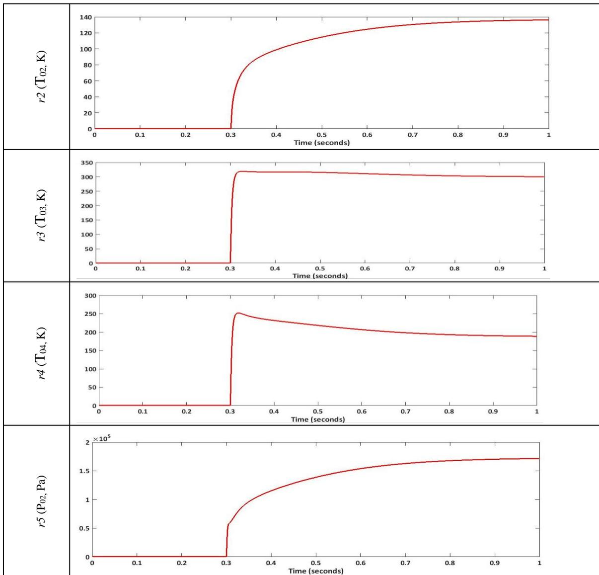
Figure 5.8(a): Residual plots ( $r2$  to  $r5$ ) in case of  $f2b$  (+50% in  $\dot{m}f$ )
