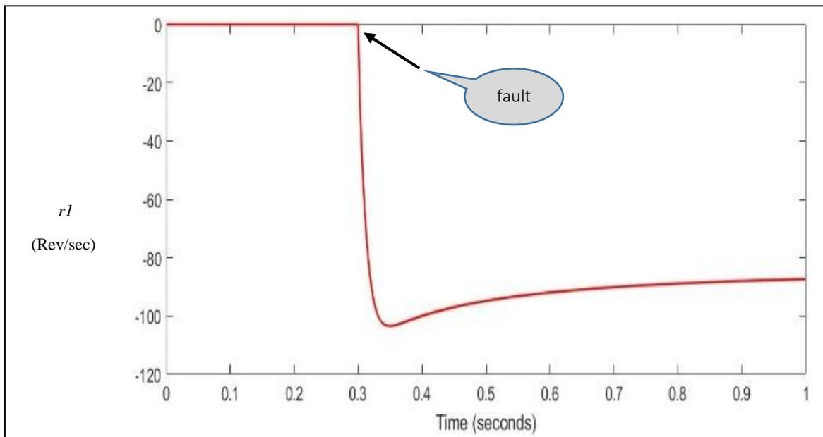
Figure 5.9: Results of residual plots ( $r1$ ) in case of  $f3$  (-26.9% in  $\eta_c$ )
