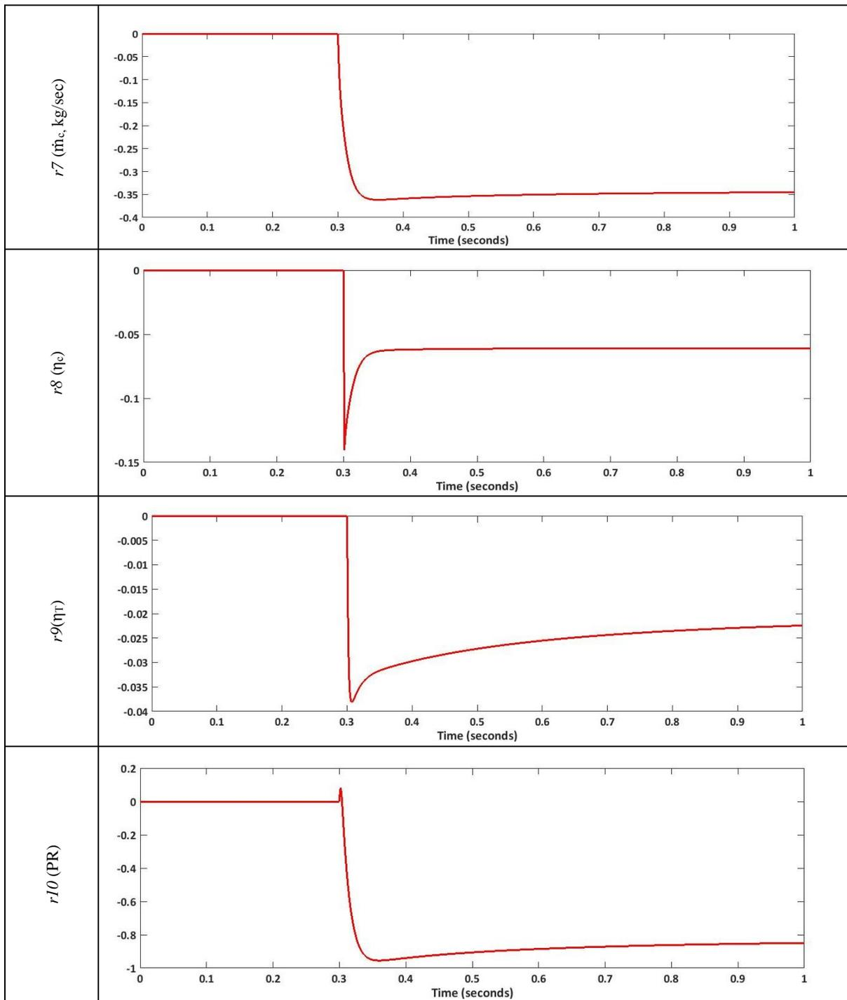
Figure 5.10(b): Results of residual plots ( $r7$  to  $r10$ ) in case of  $f3$  (-26.9% in  $\eta_c$ )
