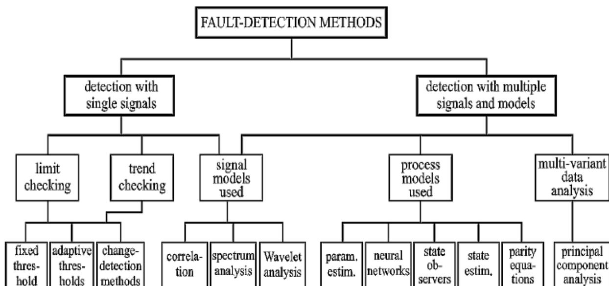
Figure 2.2: Survey of fault detection methods with signal models (Isermann, 2006)
