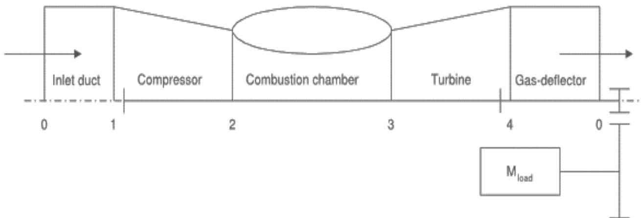
Figure 3.1: Main Parts of a gas turbine Engine (Ailer, Santa and Szederkényi, 2001)
