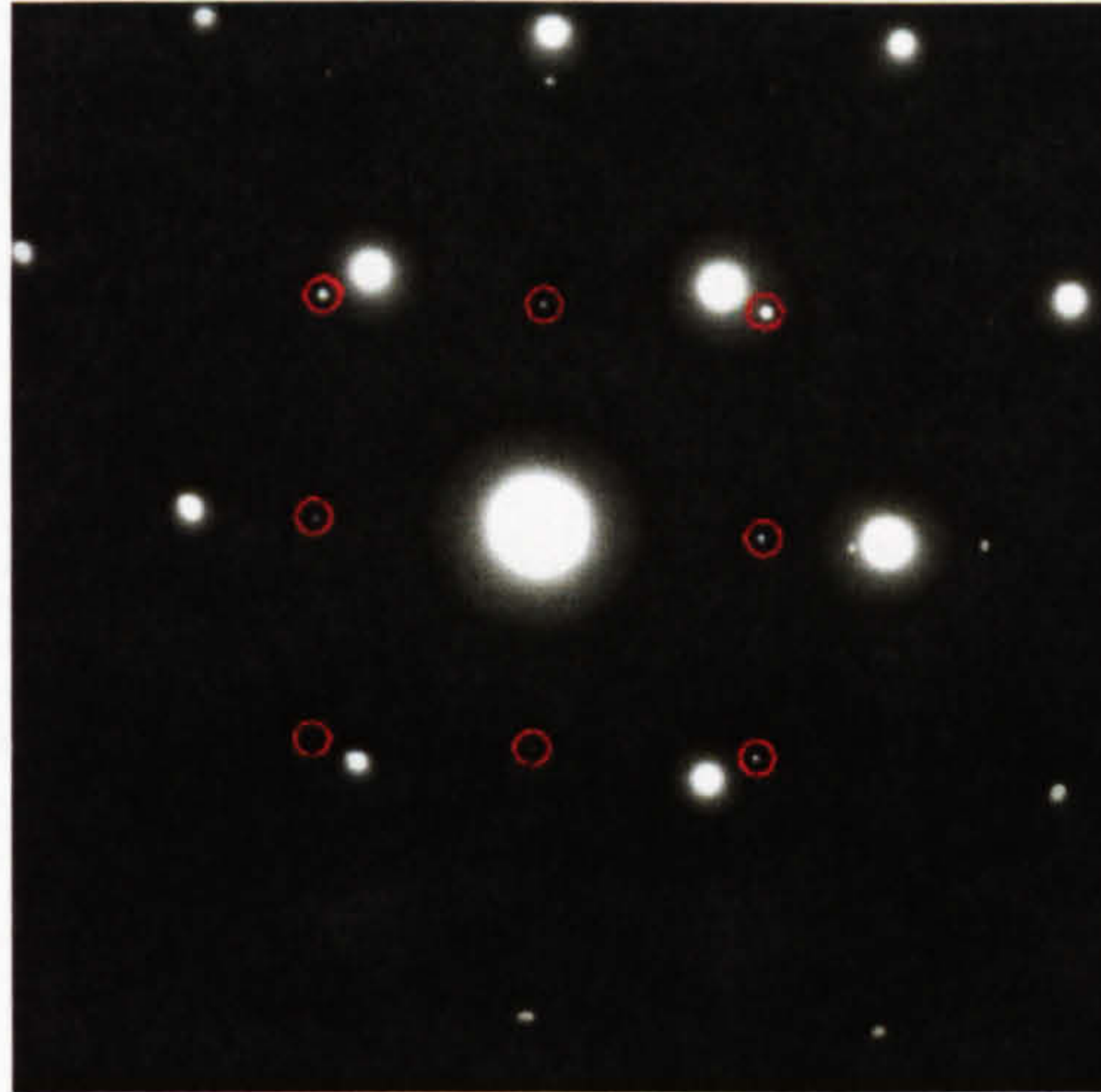
Figure 4.1: [100] Diffraction pattern from the edge of an \text{Mg}_2\text{Si} precipitate (circled in red) including the [110] diffraction pattern from aluminium.
