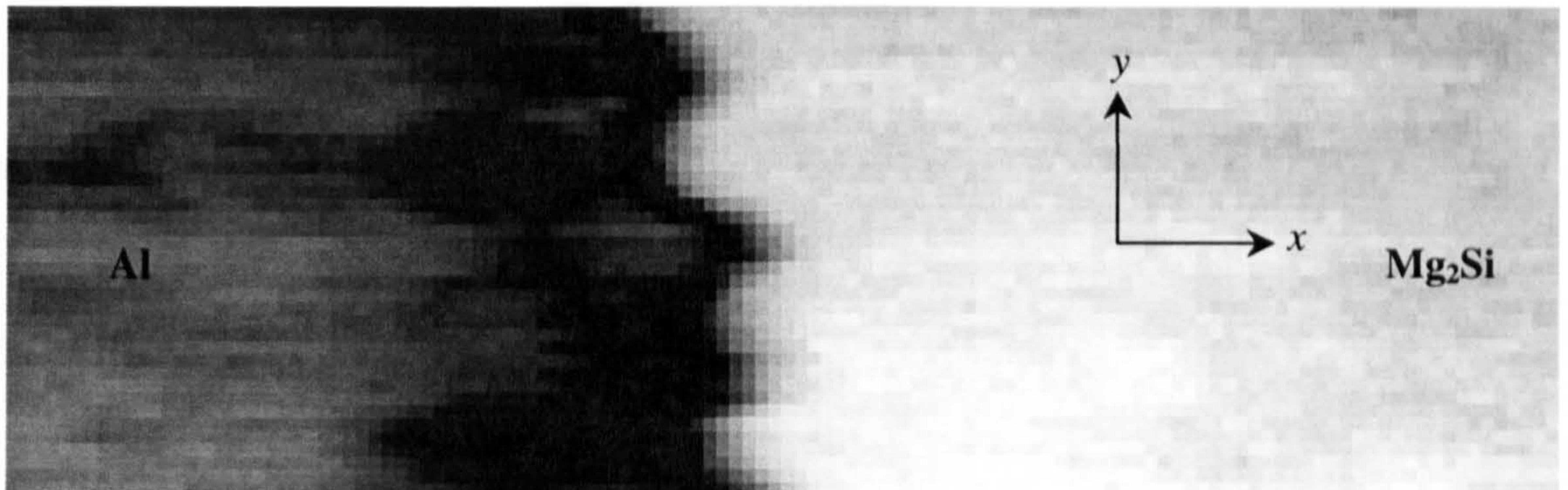
Figure 6.11: Spectrum image of an Al/Mg 2 Si interface. Intensity in each pixel is calculated using the number of counts in the corresponding zero loss peak for that pixel. This spectrum image corresponds to an area of dimensions 34nm x 11nm.
