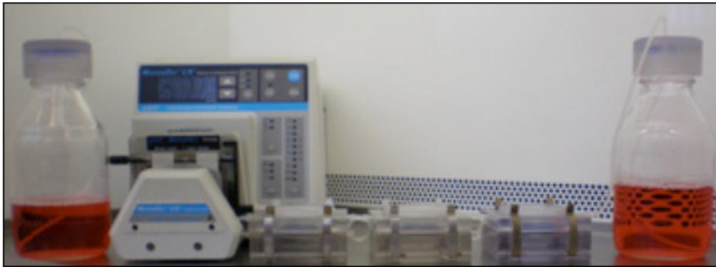
**Figure 2.2 The bioreactor.** The flow system bioreactor used in this study contained medium reservoirs (one fresh media, one used media) at both ends of the system, three cassettes of tissue containers and a peristaltic pump which generated 0.5 ml/min medium flow-rate.
