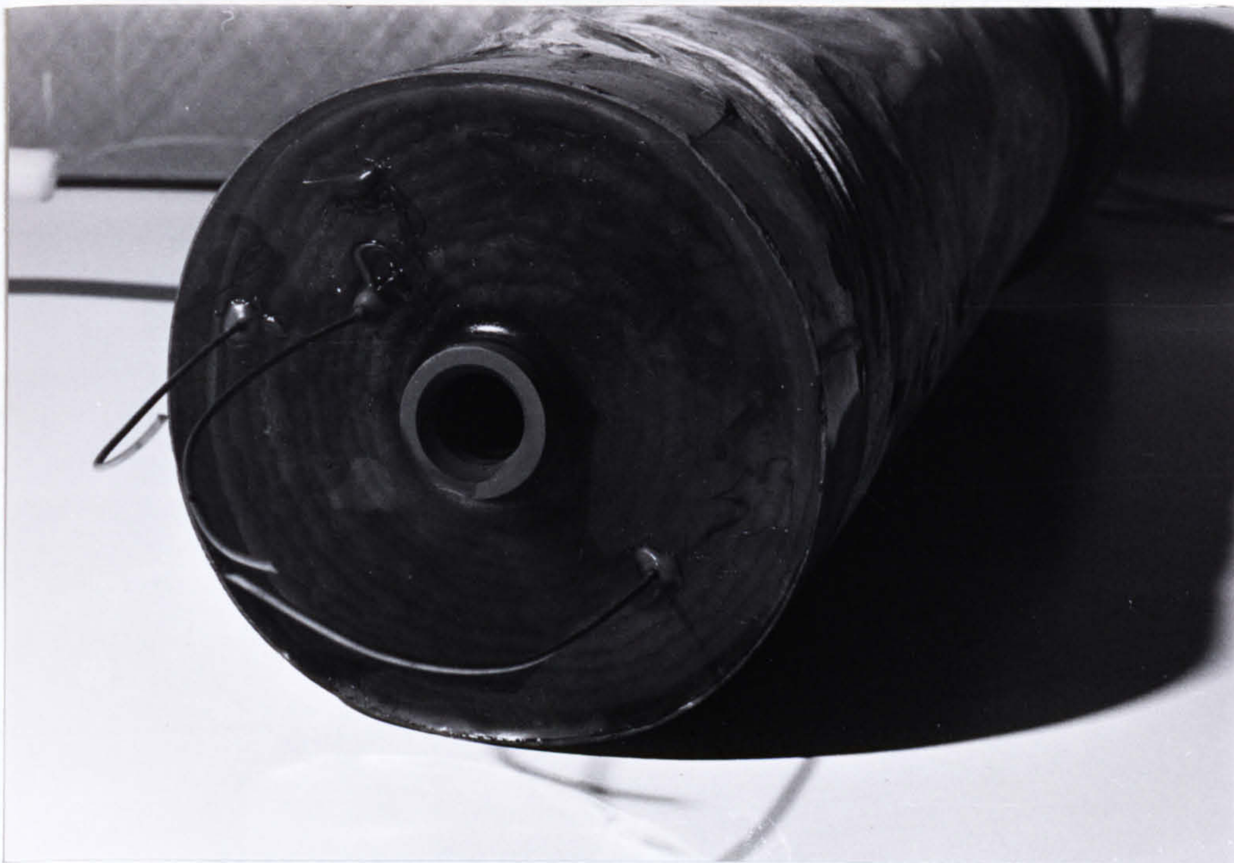
Fig. 6.3 Picture showing the pressure tapings on B-9 membrane closed end tube.
