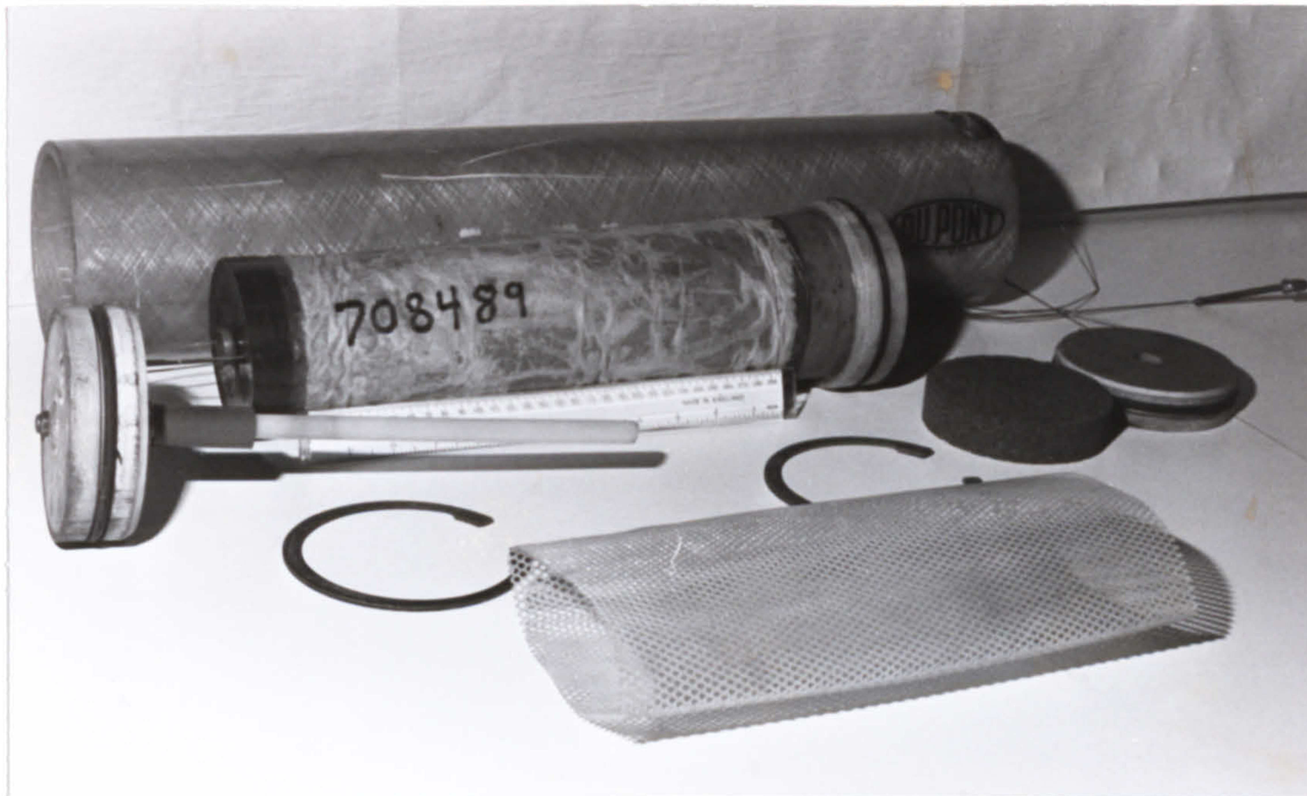
Fig. 6.1 The elements of B-9 Hollow Fibre Membrane
